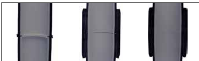
Heated element butt welding
