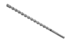
TE-Y (SDS Max) DRILL BIT Diameter Range: 12 mm - 40 mm Length Range: 320 mm-540 mm No. of Cutting Edges: 2 Applications: Anchor & rebar installation.
