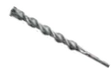
TE-YX (SDS Max) DRILL BIT Diameter Range: 12 mm - 35 mm Length Range: 320 mm-720 mm No. of Cutting Edges: 4-6 Applications: Anchor & rebar drilling.
